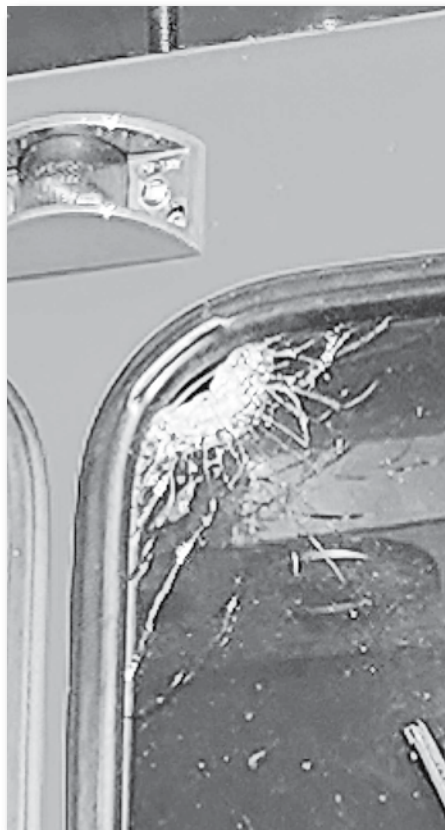
Mammoth Fire Engine 663 was struck by a discharged ammunition round during a structure fire.
