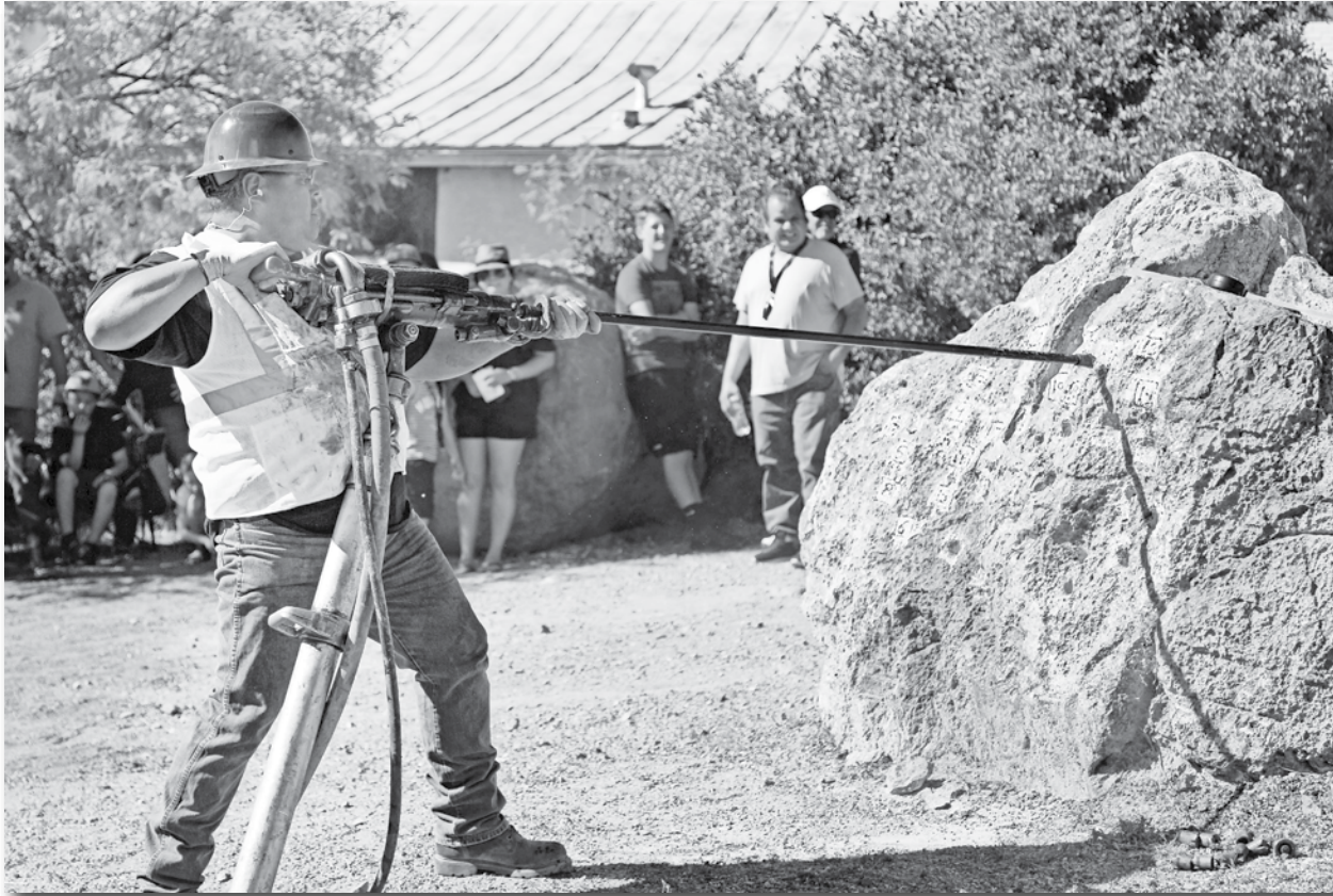
Jackleg Drilling during the Mining Competition at a previous year's Apache Leap Mining Festival.
